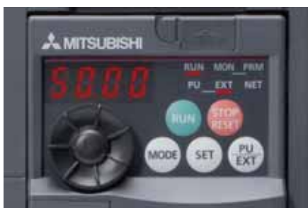
The installed Multi User Panel with the Digital Dial
