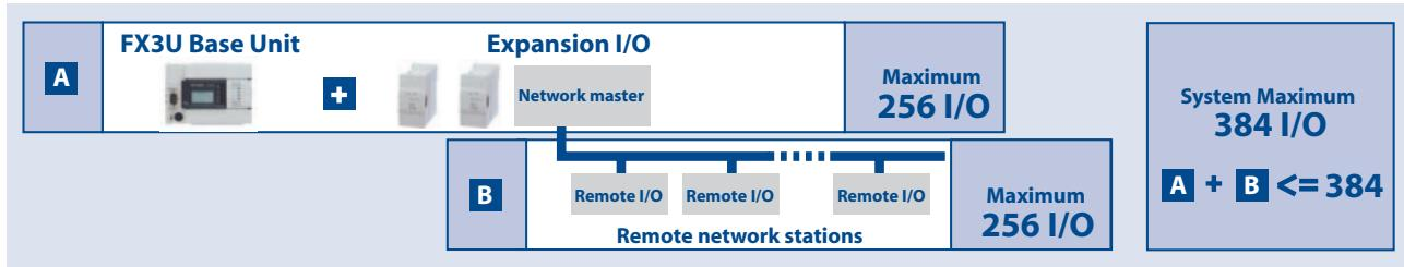
FX3U provides additional I/O and networking capacity.
